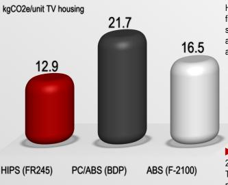
▶ HIPS (FR245): HIPS (FR245) consists of a blend of inputs including High Impact Polystyrene (HIPS, 81% of inputs) a widely used plastic, the fire retardant FR245 (15%) which is supplied from ICL-IP's Ramat Hovav site in Israel, and antimony trioxide (4%) which is used for its properties as a flame retardant synergist. These inputs are blended to produce granules and moulded into the required form using an injection moulder.
